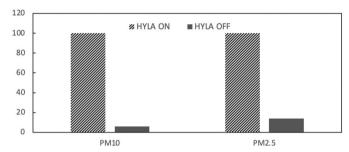
**Fig. 3.** Relative efficiency of the HYLA air purifier in reducing PM10 and PM.2 with respect to natural particulate matter deposition.
